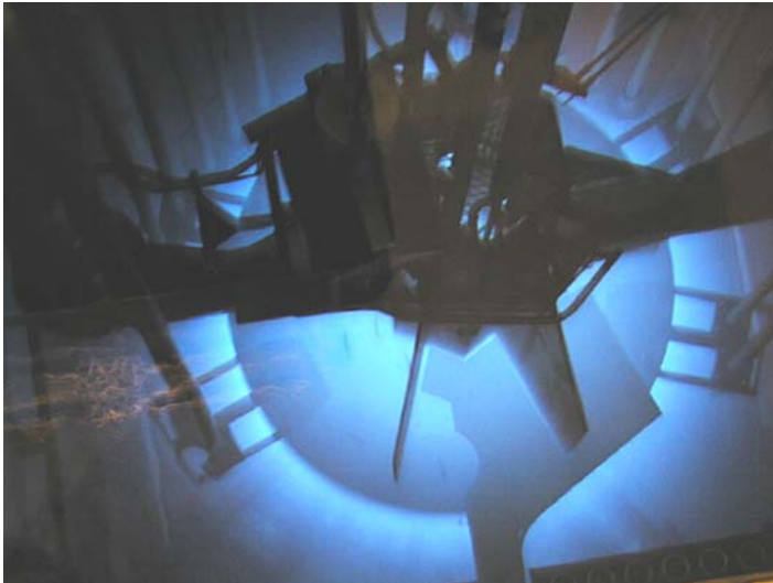
MAPLE 1 irradiating medical isotope targets at 50% power
