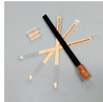
Nordion has designed tape tab holders to ensure the proper dose is delivered to the alanine pellet
